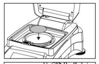
Place the empty sample pan and glass fiber pan in the pan handle. The sample pan must lie flat in the pan handle.
